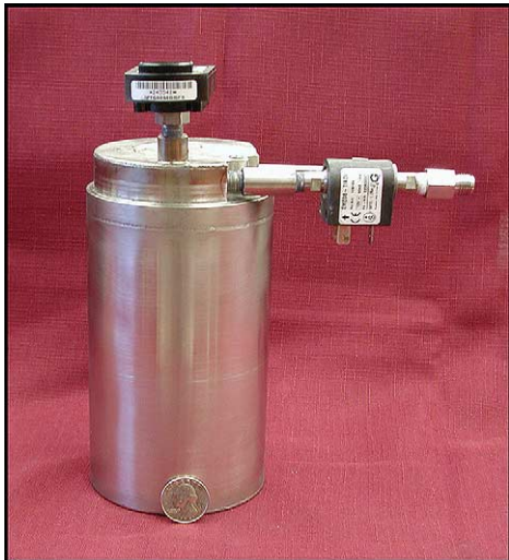
Fig. 5. Horizontal H 2 generator. The reactor, which is coiled in the lid is shown with pump, pressure sensor, and the by-product catch vessel.
