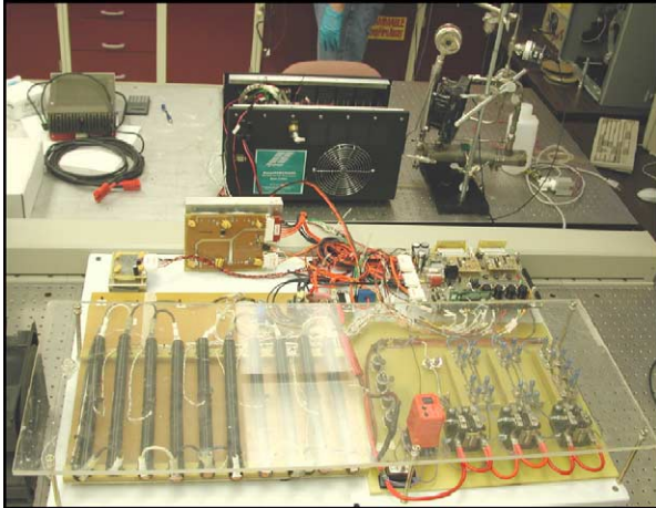
Fig. 17. Bench-top hybrid power system. The system includes the fuel cell, hydrogen generation system, transient handler, controller, and light bank for load.
