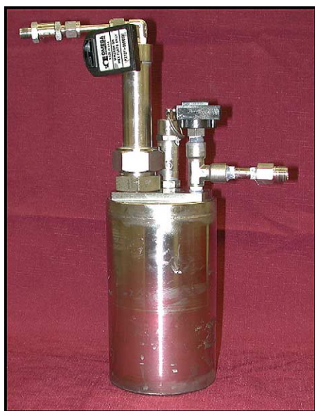
Fig. 12. Differential reactor. Shown with by-product catch vessel, pump and pressure sensor.
