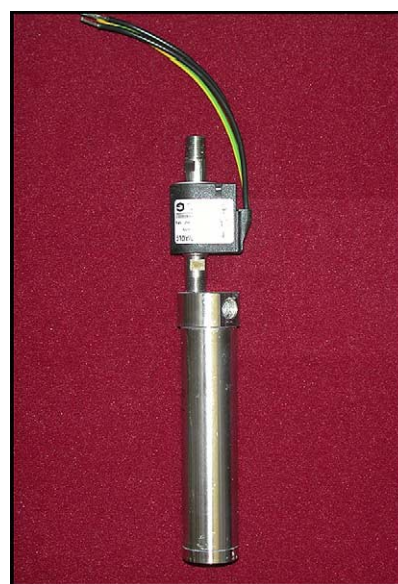
Fig. 4. Tubular H 2 generator. Stainless steel tubular generator is shown with the pump. Hydrogen and the reaction by-products exit through the bottom.
